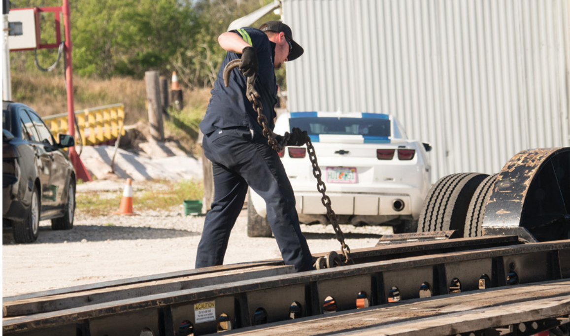
De Beradinis driver Garth Isaacson prepares tie-down chains to secure his load, a large excavator.
