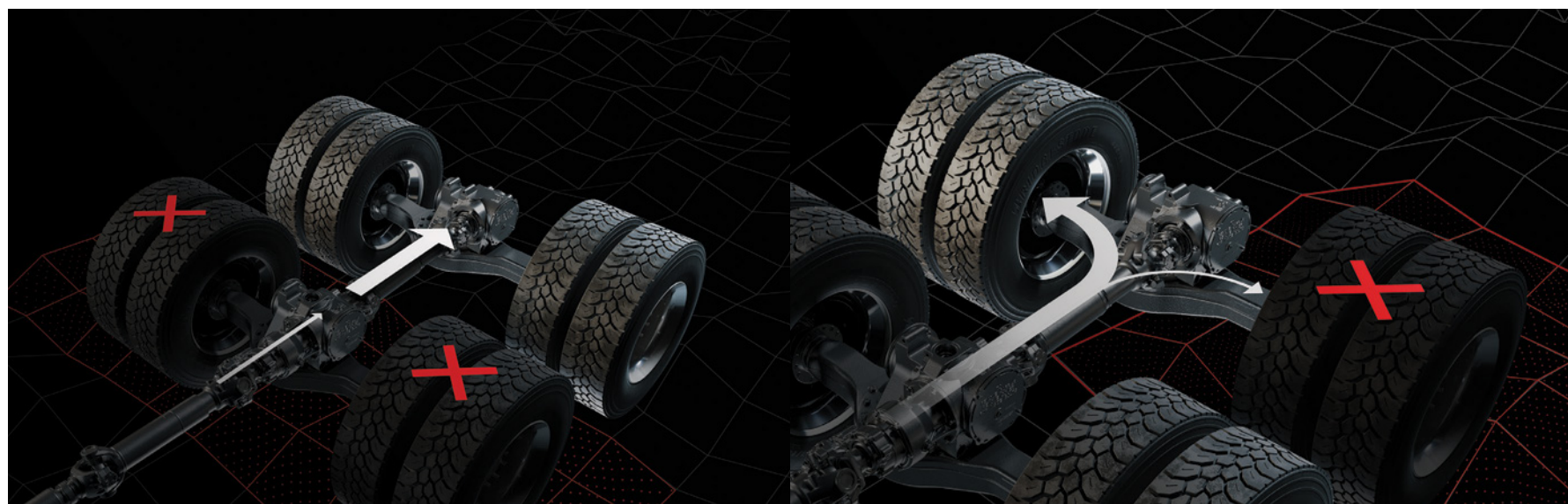
Left: Mack inter-axle power dividers automatically distribute up to 75% of torque to the axle with traction to provide power where it's needed.
